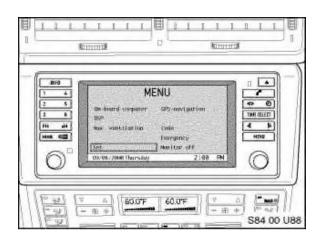
The "Wide screen" on-board monitor display (6.5" diagonal measurement) has an aspect ratio 16:9.
