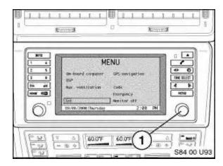
Use "<" & ">" keys to scroll through various function, and preset station keys (1-6) to select new settings (not all functions can be changed).
