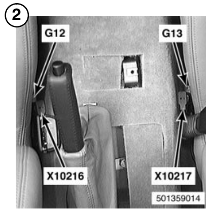
G12 DRIVER'S SIDE PYROTECHNICAL BELT TENSIONER G13 PASSENGER'S SIDE PYROTECHNICAL BELT TENSIONER X10216 X10217 501359014
