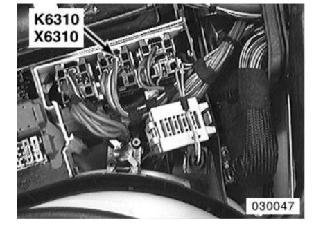
rear RH side of engine compartment in E-Box
