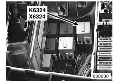
rear RH side of engine compartment in E-Box under control modules
