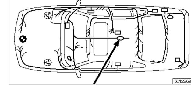
connector in wiring loom under rear of center console ahead of ABS plug connector
