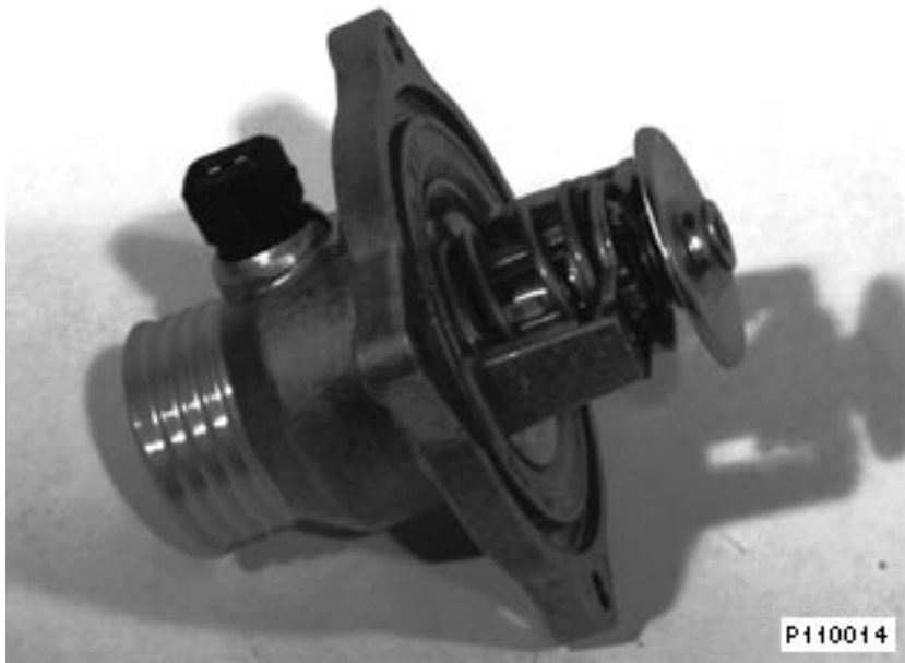
Characteristic map thermostat with electrical connection for heating element
