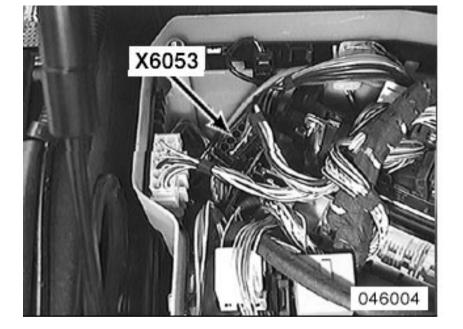
X6053 In-line connector (12-pin, Black), Engine wiring harness
