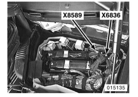
rear LH side of engine compartment in E-Box
