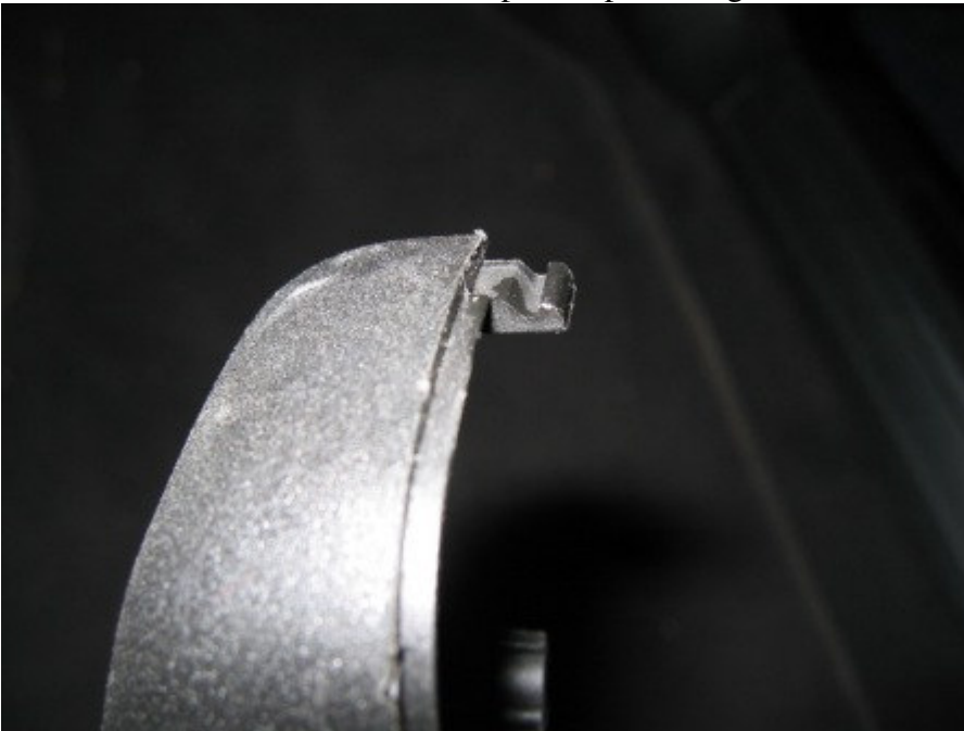
Picture2: Tabs on the cover that keep the 2 pieces together
