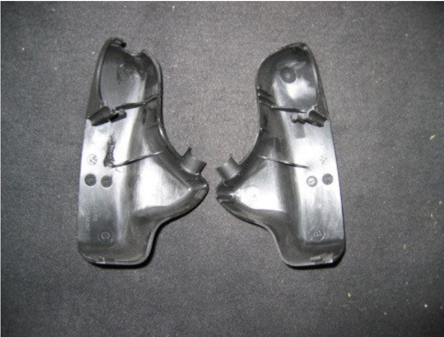
Picture1: Covers behind the rearview mirror that sit over the rain sensor.
