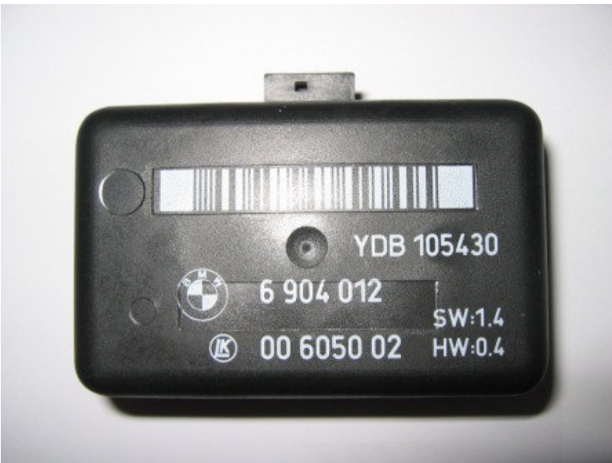
Picture6: The back view of the new rain sensor
