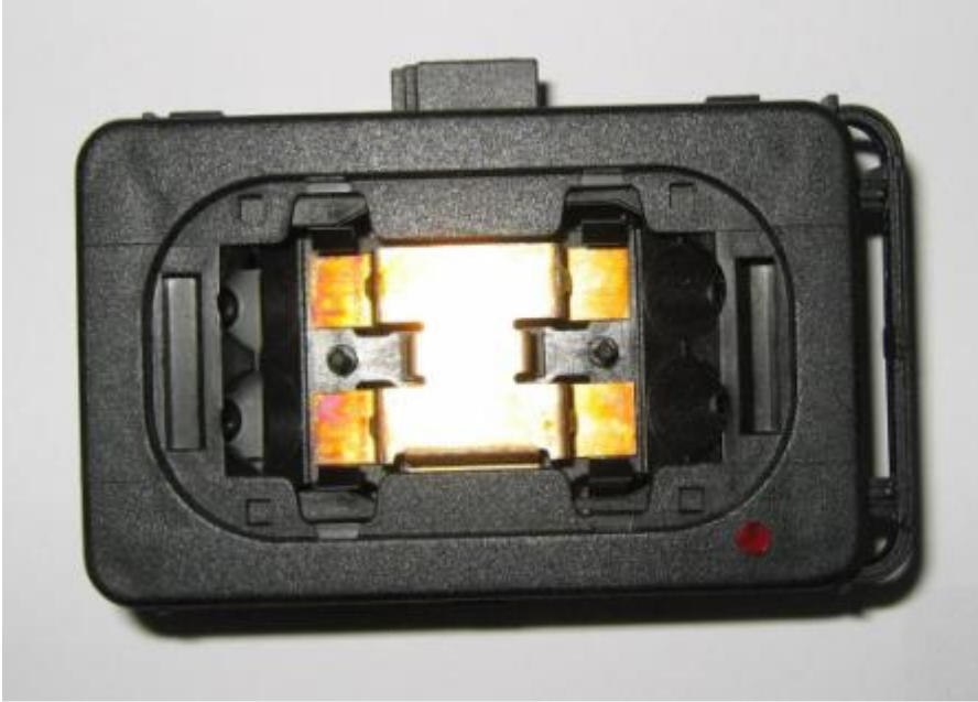
Picture3: Picture of the actual rain sensor that is being replaced
