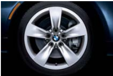
□ 18 x 8.0 Star Spoke (Style 246) cast alloy wheels with 245/40R-18 run-flat performance tires. 3 (incl. in 528i Sport Package, opt. with 528xi Sport Package; spare is a space-saver wheel and tire)
