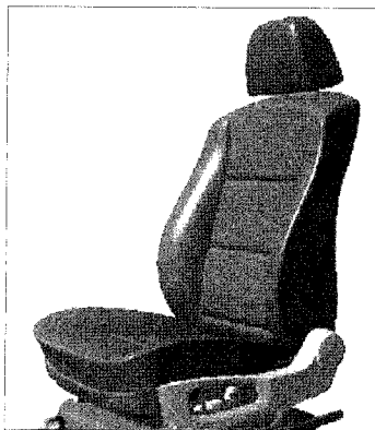
The standard front seats in all models incorporate 10-way power adjustment, with their controls (including memory) on the seats' outboard edges.
