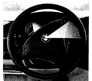
...and here the motion required for the same steering of the front wheels at higher speeds.
