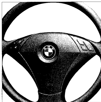
For the first time in the 5 Series, a 3-spoke steering wheel is standard in all models. Once again it is tilt/telescopically power-adjustable (now with faster adjustment), and when the key is removed the wheel rises to its highest position for ease of exit and entry.
