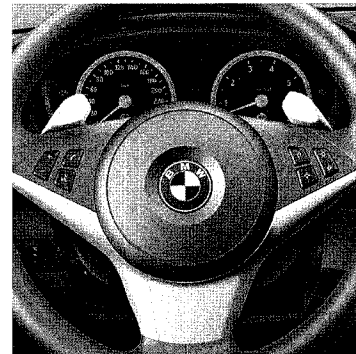
Shift "paddles" on the steering wheel: thanks to Active Steering, now more convenient.
