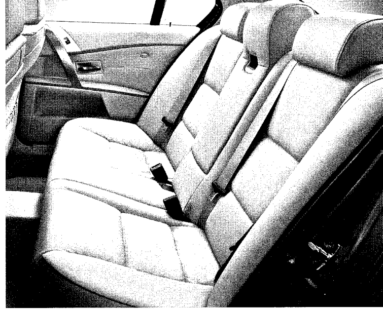
Newly designed rear-seat structure provides standard or fold-down seats with no variation of the body structure itself.
