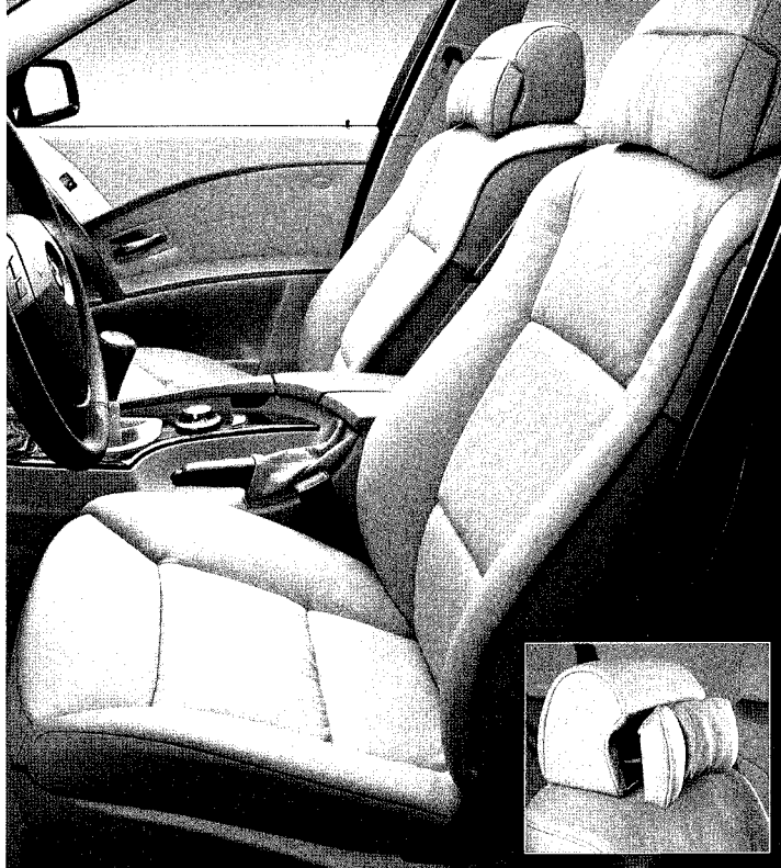
16-way power Comfort front seats were available in the previous 5 Series; now this feature appears in evolved form, with 20-way power adjustment, memory for both driver
