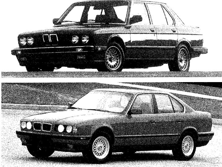
With the 2nd-generation 5 Series (E28, top), BMW essentially "re-skinned" the 1st-generation body, but also incorporated many engineering improvements. This is a 1987 535is, the "s" meaning a sport version.
