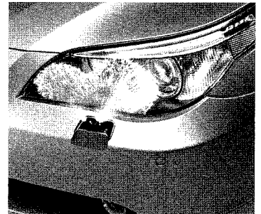
New retracting headlight washers are part of the Cold Weather Package.
