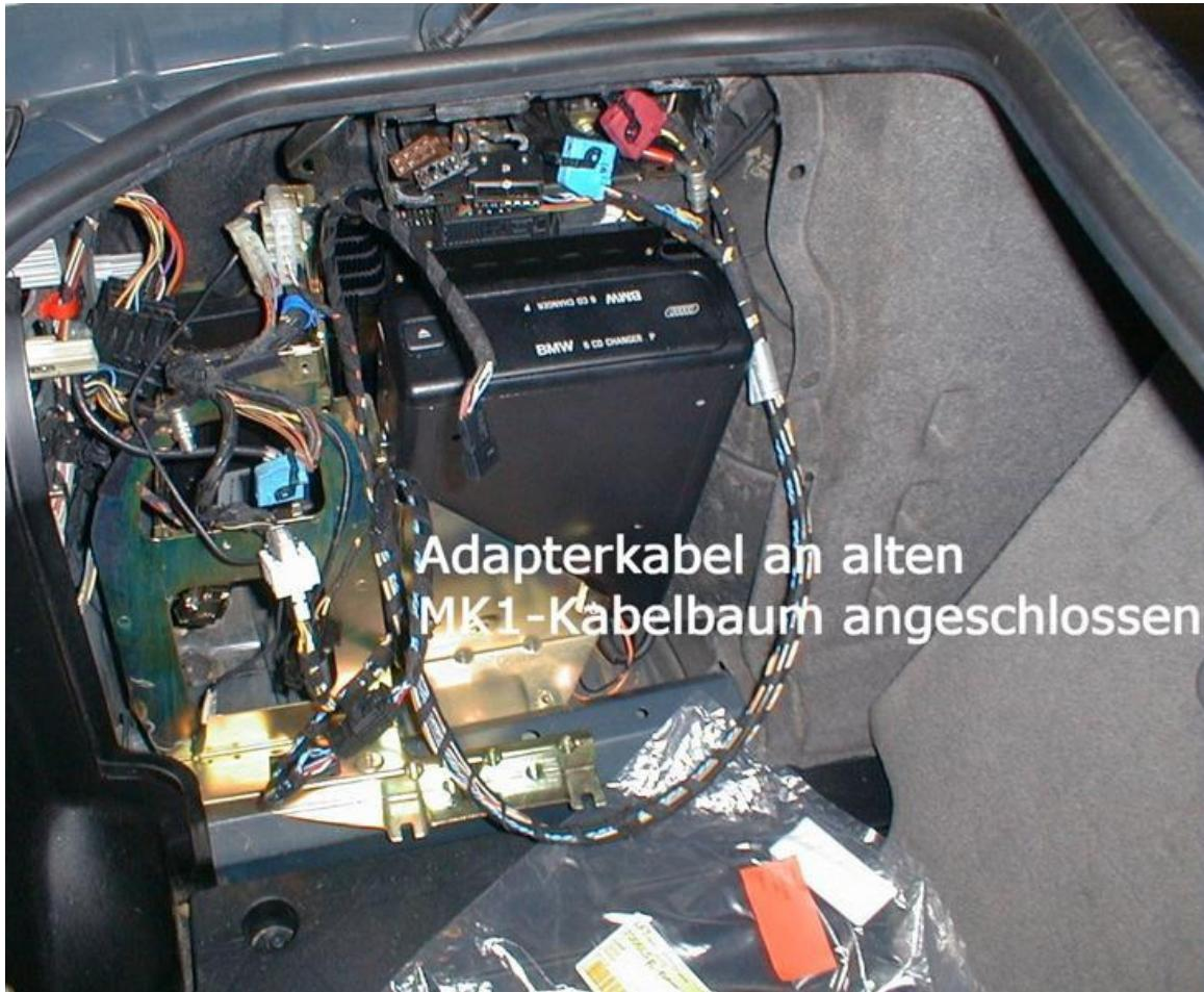
On the left you can see the brown and black connector (MK I or old MK II) On the right are the new connectors (blue and purple) The cable that runs all around the CD Changer is the adaptor Cable from BMW. Part No.: 61 1 28 381 219
